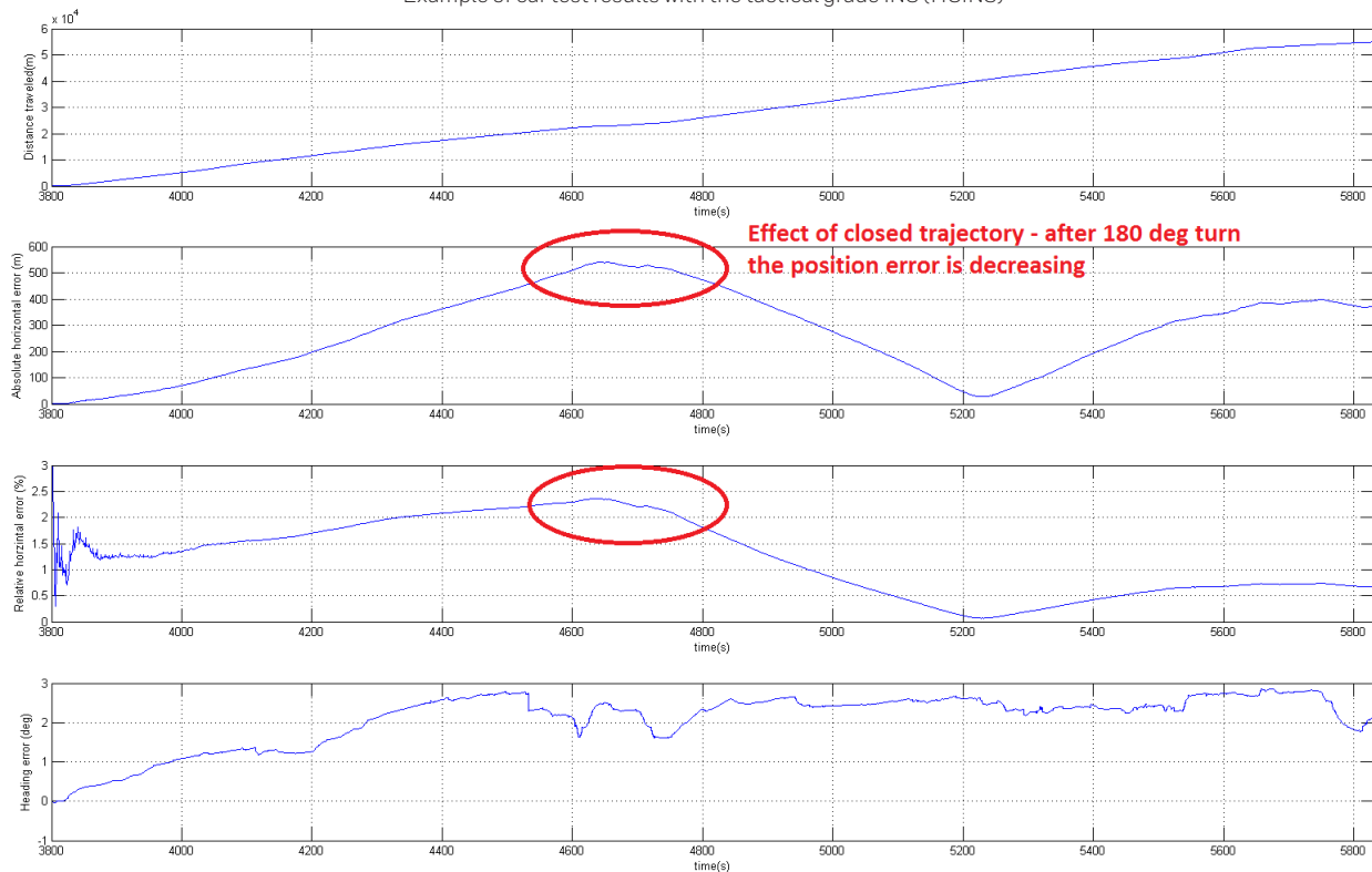
Example of car test results with the tactical grade INS (HCINS)
